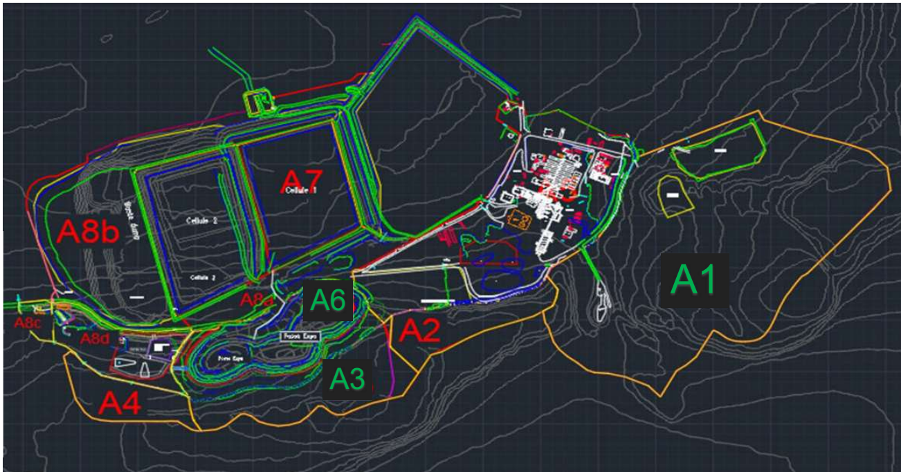
Figure 1: Catchment Areas at the Expo Site (Catchments in Green do not Report to the MCP)
