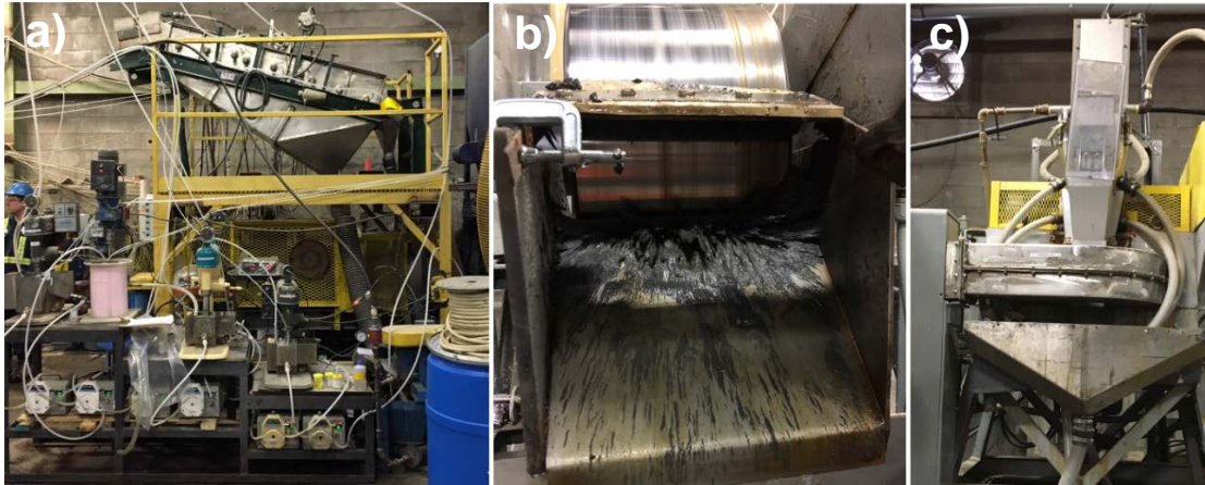
Figure 12-11: Pilot Plant a) Grinding, b) LIMS, and c) WHIMS
