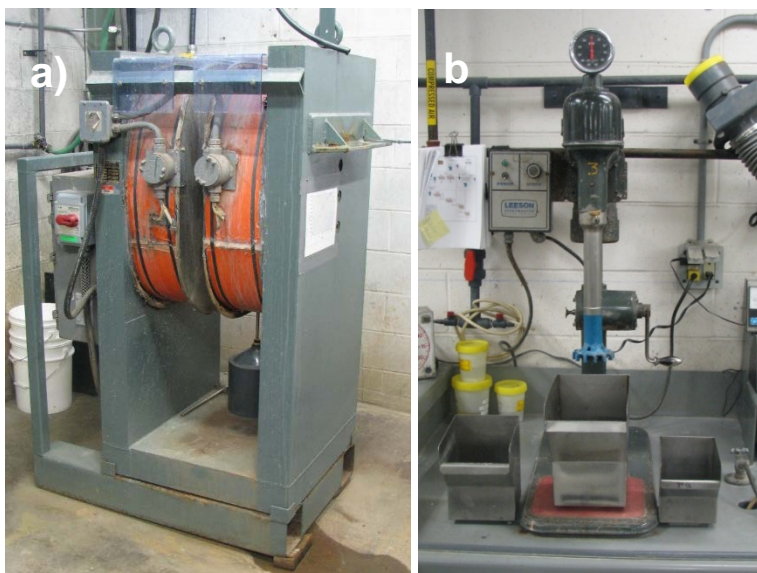
Figure 12-7: Batch Testing Equipment: a) WHIMS, and b) Flotation Machine and Cells
