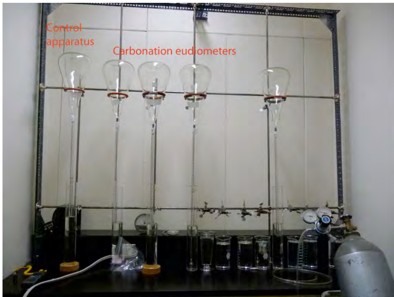
Fig. 20: Five 4L eudiometers. The apparatus seen on the left is loaded with quartz and the others contain experimental samples.
