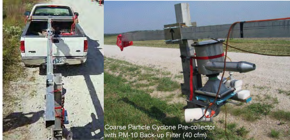
Figure 5.1 Mobile Dust Emission Monitor by MRI [2]
