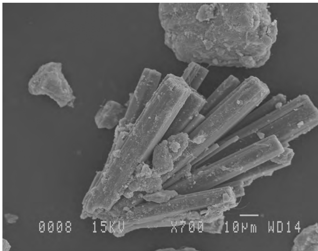
Fig. 42: RN4b-FT184F : Bundle of acicular carbonate crystals among serpentine grains.
