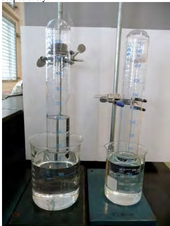
Fig. 19: Two 500 mL eudiometers. The left eudiometer contains a sample whereas the control apparatus loaded with quartz and water is to the right.
