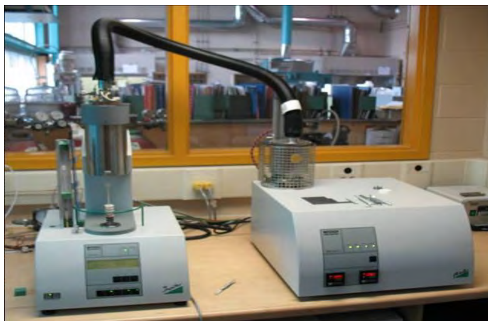
Figure 2: The Netzsch Jupiter STA 449C Thermal Analyser (open position) and the Netzsch Aeolos 403C Mass Spectrometer.
