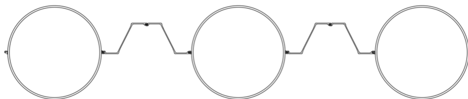
Figure 4.5.1 : Mur combiné 1 219 dia. × 22,225 mm / AZ 26-700
