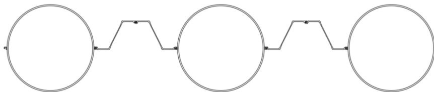
Figure 4.4.5 : Mur combiné 1 219 dia. × 19,05 mm / AZ 26-700
