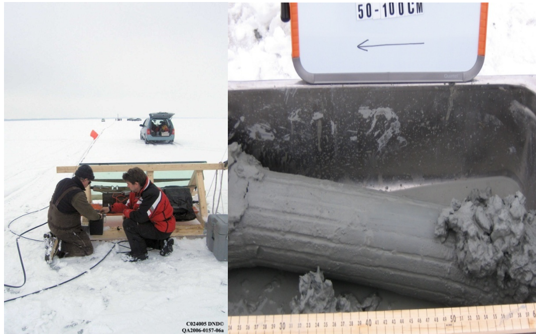
Figure 109: Setting up remote control drill and example of sediment before clearing by UXO technician
