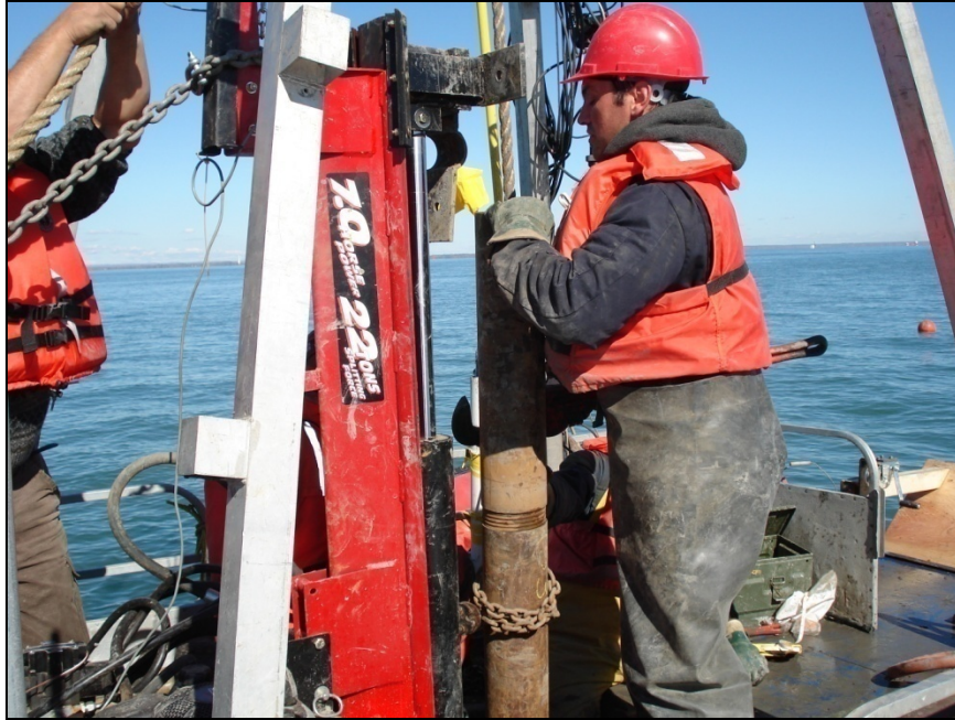
Figure 111: Drilling Rig (modified from an hydraulic wood splitter)
