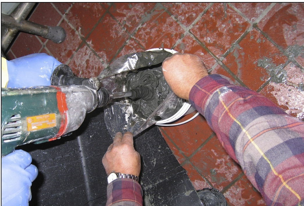
Figure 112: Mixing a 3L sample using a stainless steel mixer in an electric drill
