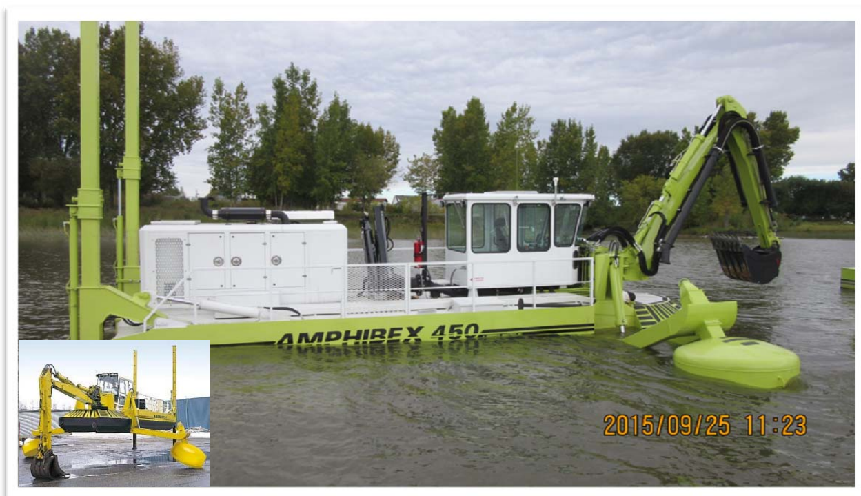
Figure 3.4 Drague hydraulique de type amphibie
