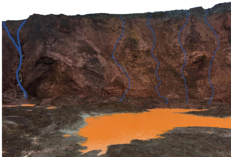
Photo 8 : Open Pit - North Wall - "Major" Water inflow in NW corner and smaller inflows on north wall
