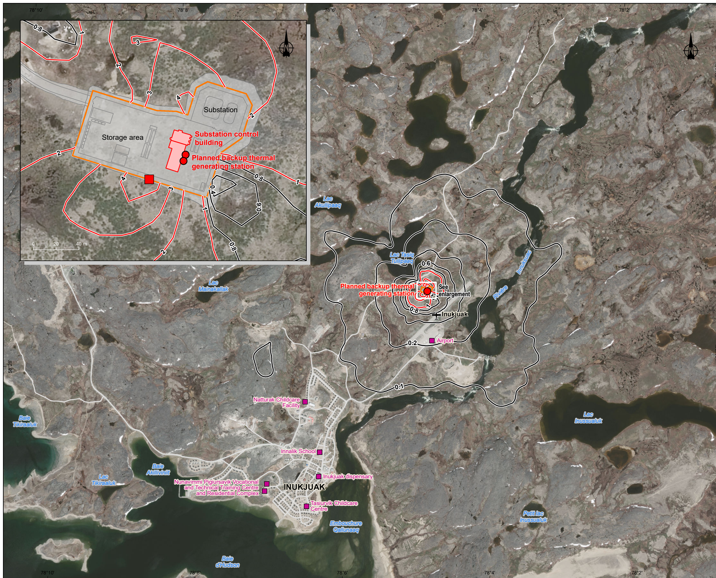
Inukjuak backup thermal generating station Maximum of the annual 98th percentiles of the maximum hourly 4-minute odor concentrations calculated in the ambient air around the plant (OU/m 3 ) during continuous operation Maximum backup scenario
