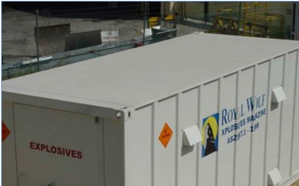
Figure 8-4 : Typical container for the safe storage of explosives
