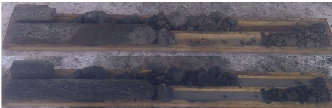
Figure 23 Rock core (dry and wet surfaces) recovered in BH21-W-08 from 16.00 to 17.90 m of depth
