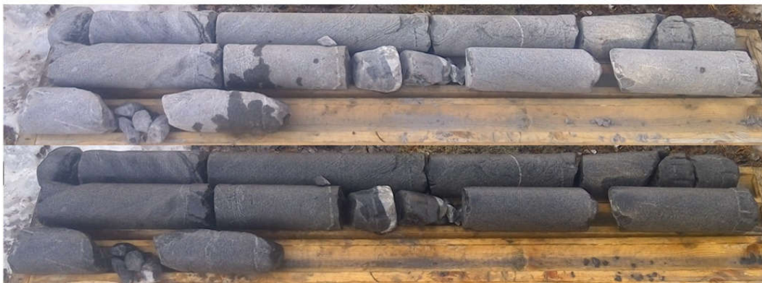
Figure 15 Rock core (dry and wet surfaces) recovered in BH21-O-06 from 11.53 to 13.15 m of depth
