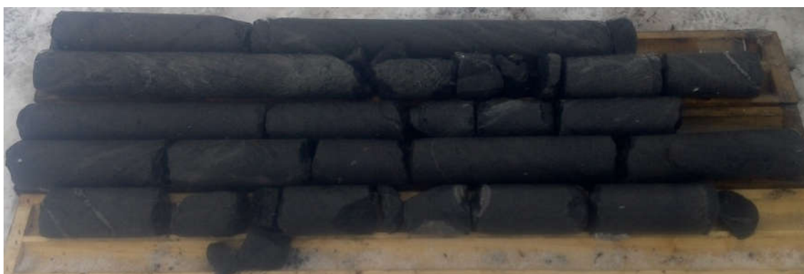
Figure 18 Rock core (dry surface) recovered in BH21-R-01 from 1.70 to 8.80 m of depth
