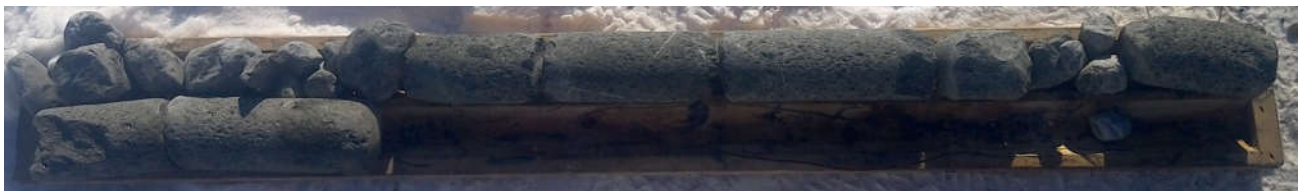
Dry rock core (RC-11) Depth from 8.15 to 11.70 m
