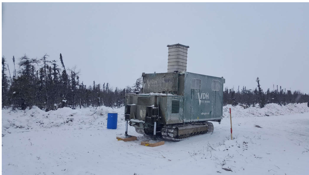
Figure 6 Crawling rig used by VDH Geo-Services for cone penetration tests
