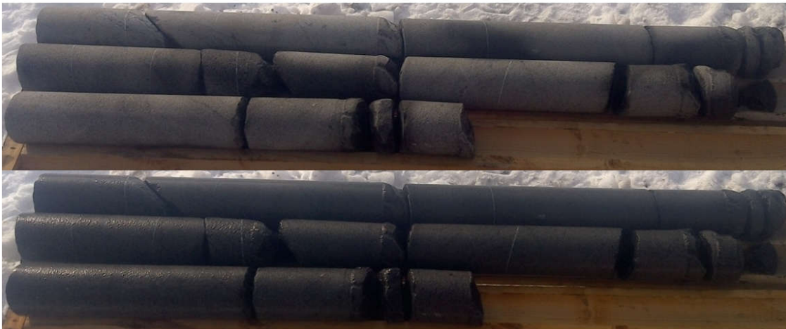
Figure 17 Rock core (dry and wet surfaces) recovered in BH21-P-04 from 2.10 to 5.85 m of depth
