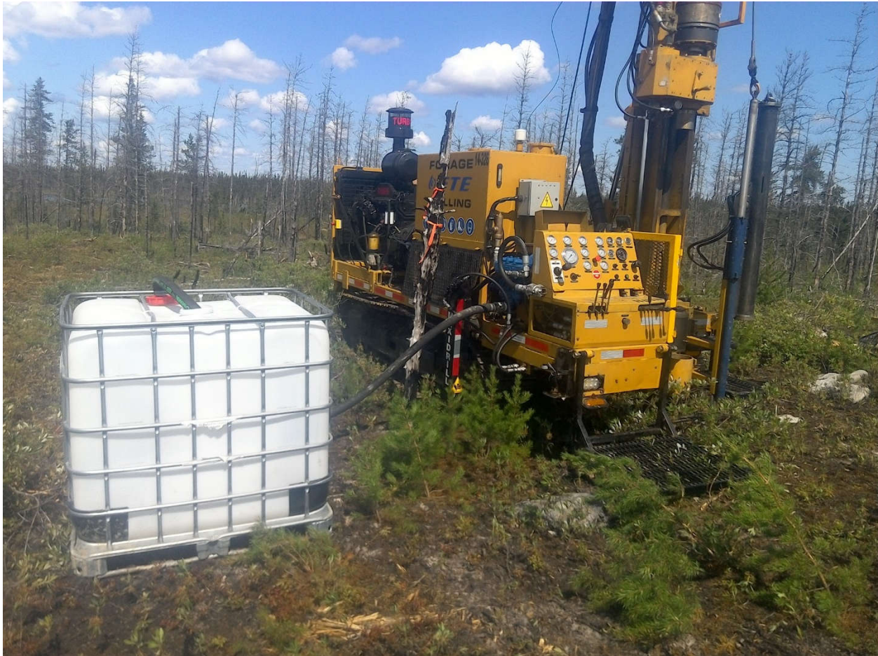
Figure 4 Maxidrill diamond drill rig
