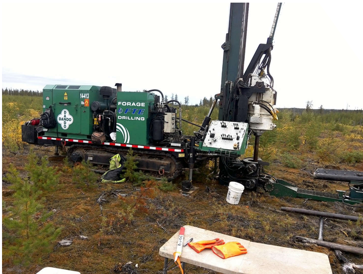
Figure 5 Dando sonic drill rig
