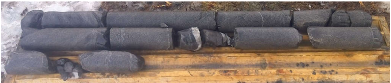
Wet rock core (RC-08) Depth from 5.15 to 9.05 m
