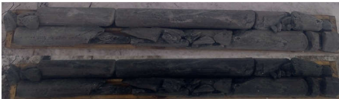
Figure 27 Rock core (dry and wet surfaces) recovered in BH21-W-09 from 3.15 to 5.70 m of depth
