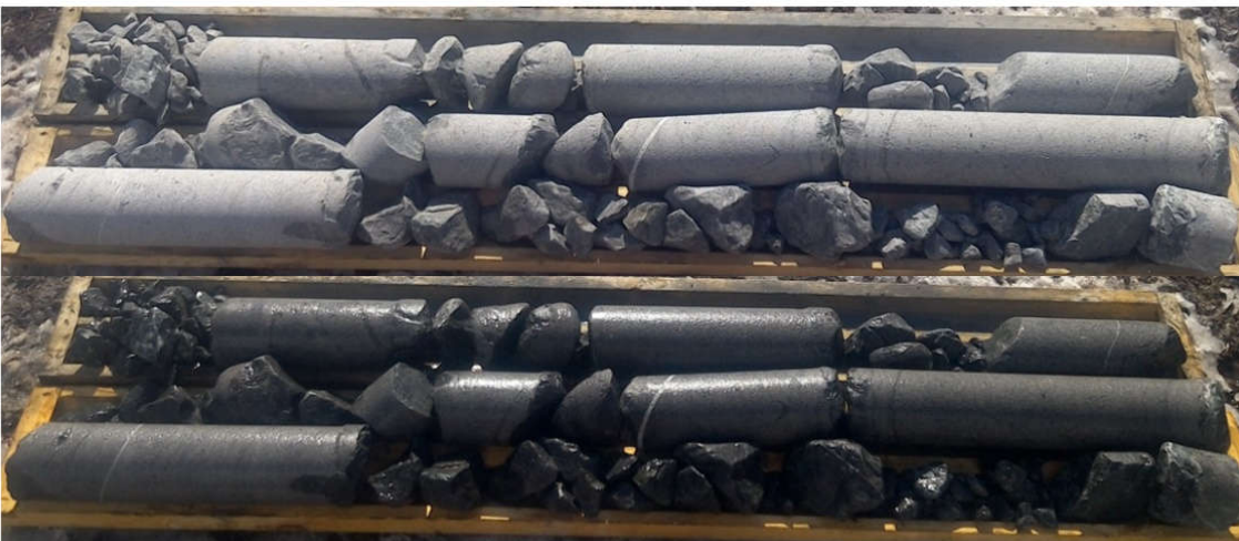
Figure 17 Rock core (dry and wet surfaces) recovered in BH21-P-04 from 2.10 to 5.85 m of depth
