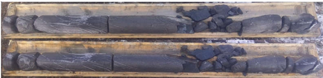
Figure 13 Rock core (dry and wet surfaces) recovered in BH21-O-04A from 7.63 to 11.30 m of depth
