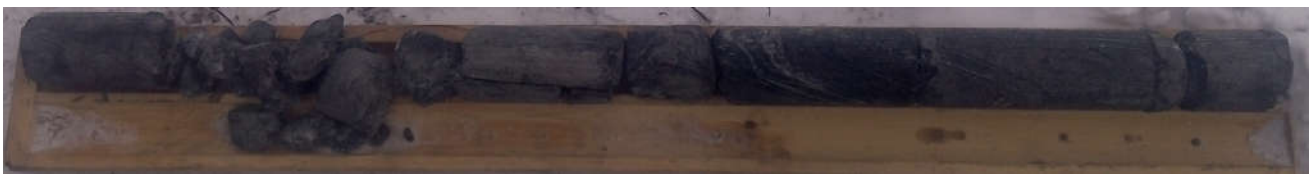
Dry rock core (RC-08) Depth from 5.85 to 7.25m
