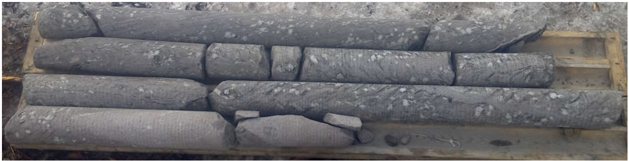
Dry rock core (RC-03) Depth from 1.00 to 5.95 m
