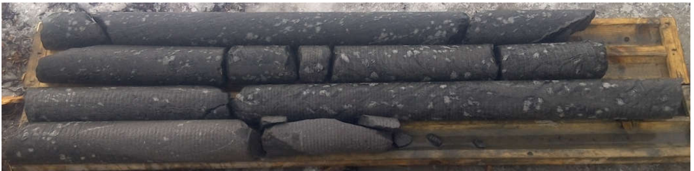
Wet rock core (RC-03) Depth from 1.00 to 5.95 m
