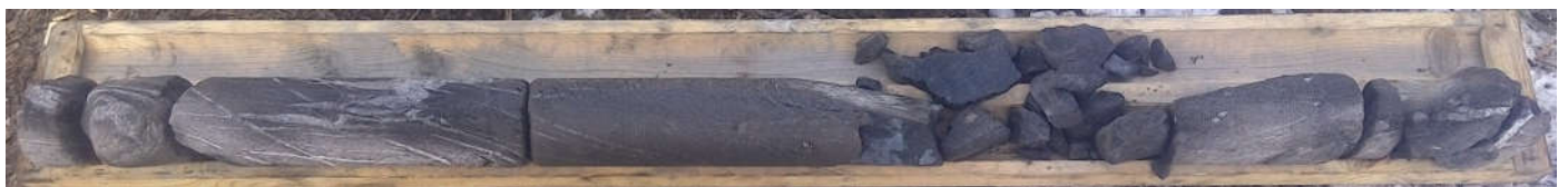
Dry rock core (RC-09) Depth from 5.25 to 6.75 m
