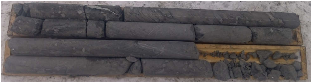
Dry rock core (RC-07) Depth from 3.55 to 9.05 m
