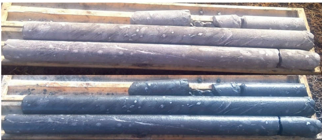
Figure 13 Rock core (dry and wet surfaces) recovered in BH21-O-04A from 7.63 to 11.30 m of depth
