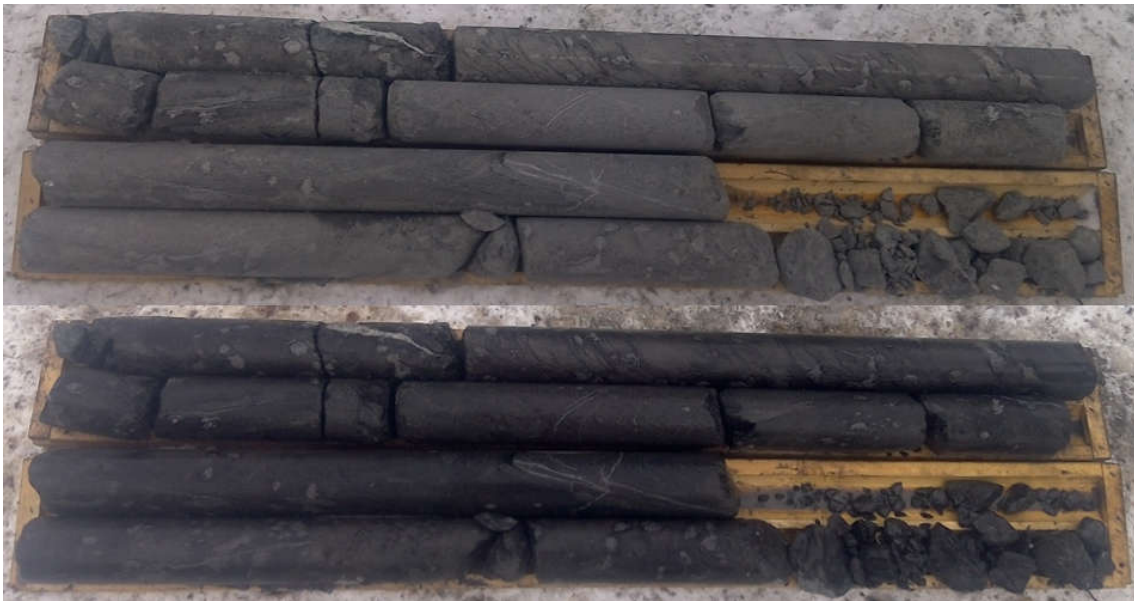
Figure 22 Rock core (dry and wet surfaces) recovered in BH21-W-04 from 6.75 to 8.85 m of depth
