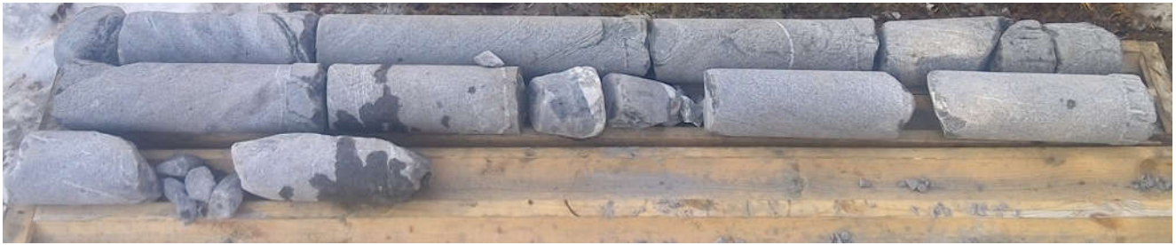
Dry rock core (RC-08) Depth from 5.15 to 9.05 m
