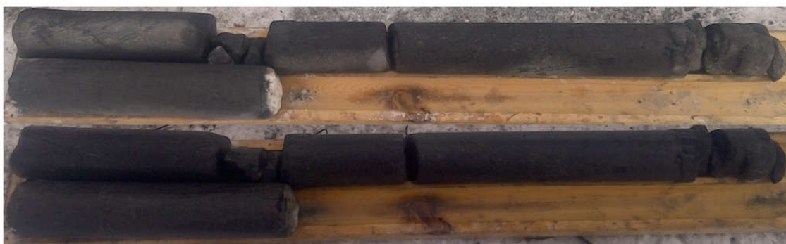
Figure 15 Rock core (dry and wet surfaces) recovered in BH21-O-06 from 11.53 to 13.15 m of depth
