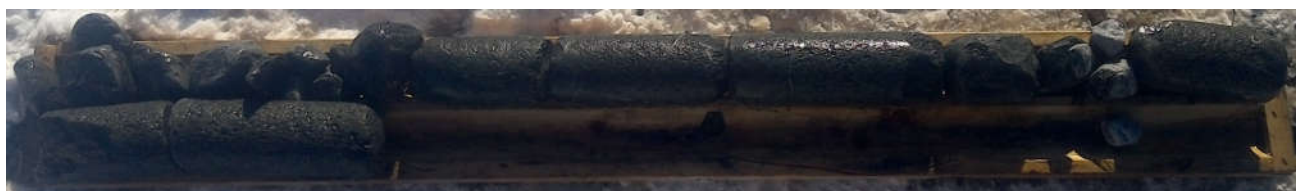
Wet rock core (RC-11) Depth from 8.15 to 11.70 m
