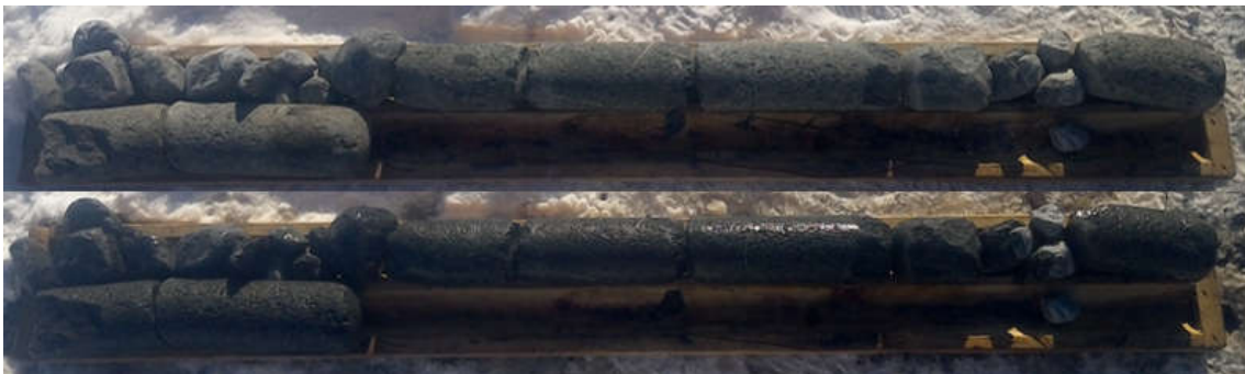
Figure 25 Rock core (dry and wet surfaces) recovered in BH21-W-05 from 5.85 to 7.25 m of depth
