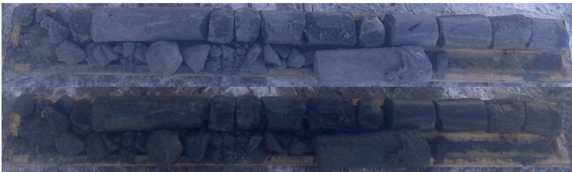
Figure 22 Rock core (dry and wet surfaces) recovered in BH21-W-04 from 6.75 to 8.85 m of depth
