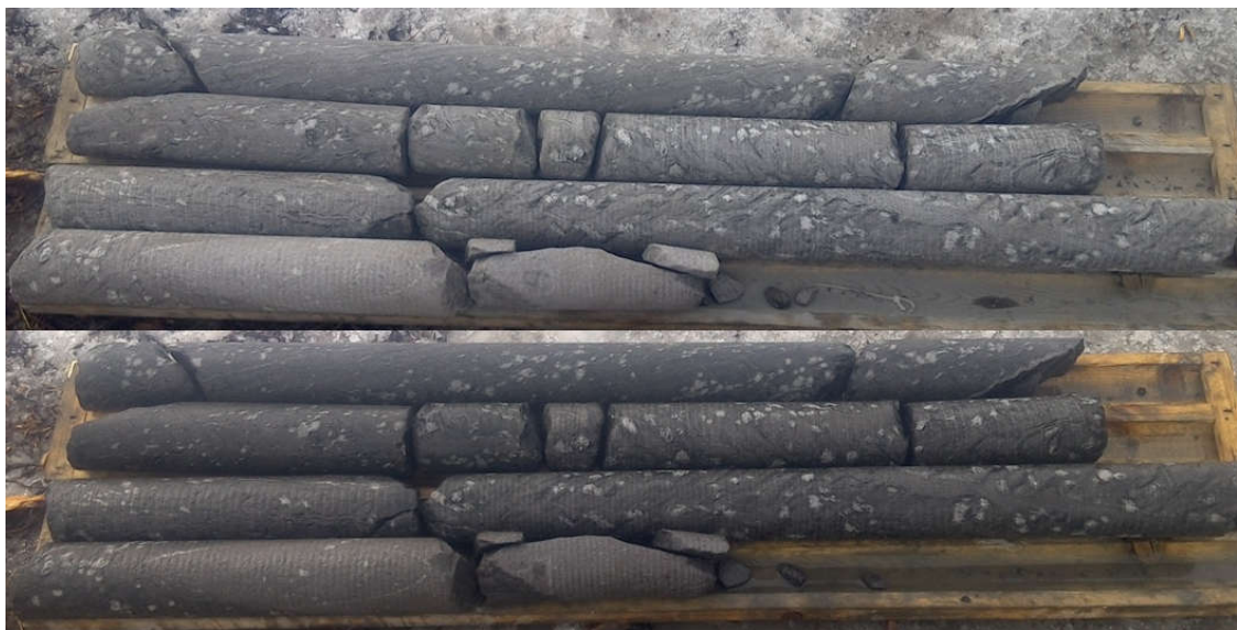
Figure 19 Rock core (dry and wet surfaces) recovered in BH21-SW-03 from 1.00 to 5.95 m of depth
