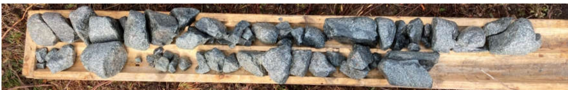
Figure 11 Rock core (dry surfaces) recovered in BH20-P-09 from 9.24 to 10.87 m of depth
