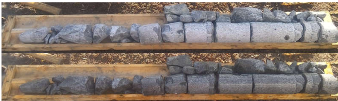
Figure 27 Rock core (dry and wet surfaces) recovered in BH21-W-09 from 3.15 to 5.70 m of depth
