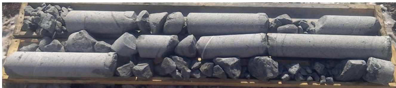
Dry rock core (RC-05) Depth from 2.10 to 5.85 m
