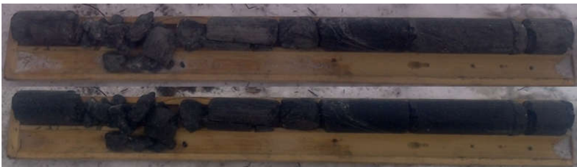
Figure 25 Rock core (dry and wet surfaces) recovered in BH21-W-05 from 5.85 to 7.25 m of depth
