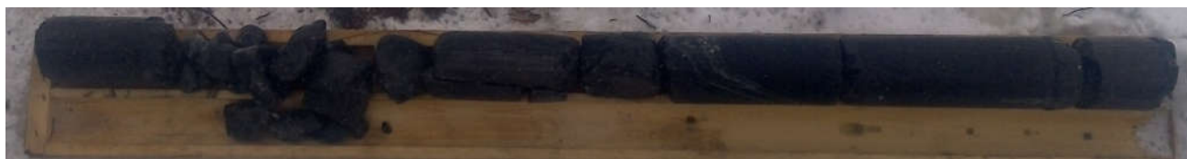
Wet rock core (RC-08) Depth from 5.85 to 7.25m
