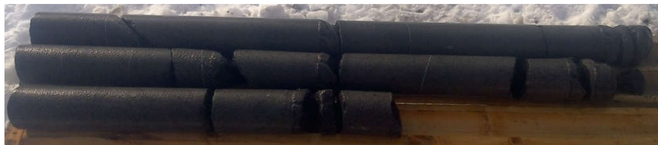
Wet rock core (RC-04) Depth from 2.09 to 5.95 m
