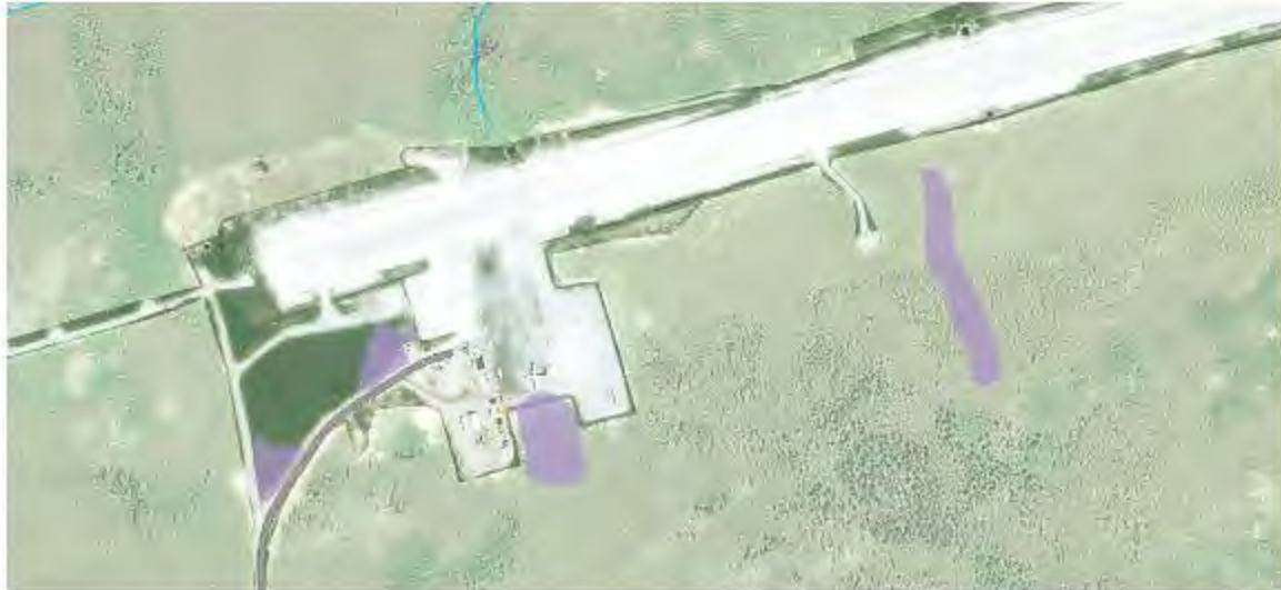
Figure 5 - Aerial photo of the airport showing the avoidance of peatlands, shown in mauve.
