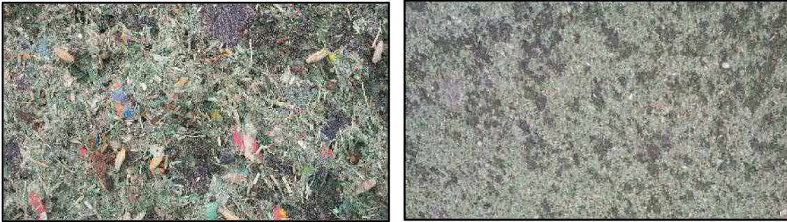
Photos 10 & 11 Close up of Hydroseed/Mulch Mix
