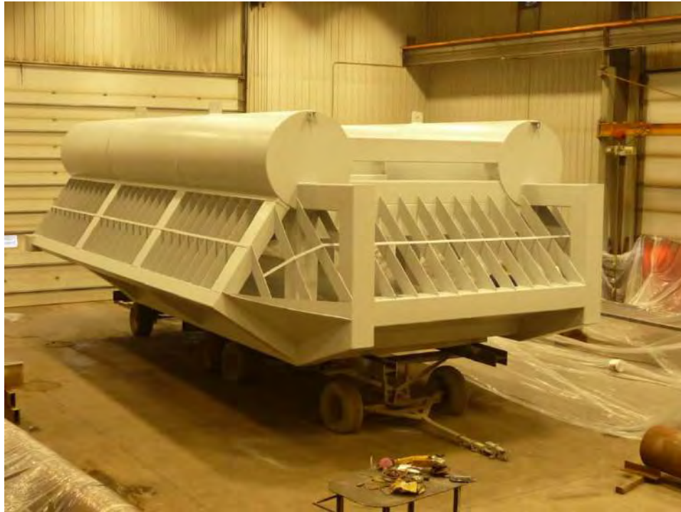
Photo 2.1: Typical Siphon Intake Structure
